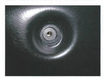
4. Bolt on the bracket together with the washer, spacer and stainless steel bolt and torque carefully. Be gentle and do not over torque!
