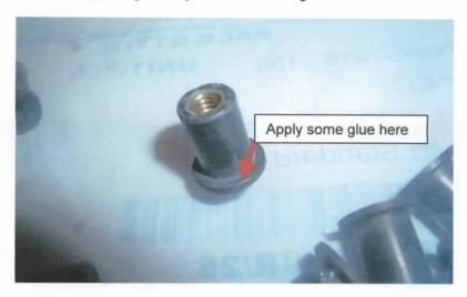
3. Install the Well Nuts to the firewall and wait to let the glue dry.
